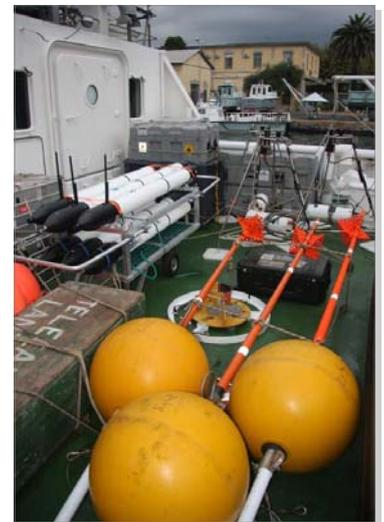
Top: A schematic of LOON, which consists of fixed (bottom-mounted) and mobile nodes. Bottom: Some of the nodes used in a CMRE experiment, including the Folaga autonomous underwater vehicles, surface marker buoys, and bottom-mounted tripod modems.
