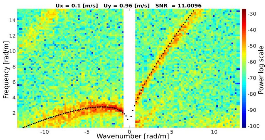
Figure 3: Wave number frequency plain along the main flow direction of the Elbe River retrieved from a box of 20 m x 20 m in the main flow of the Elbe River (yellow square indicated in Figure 2).
