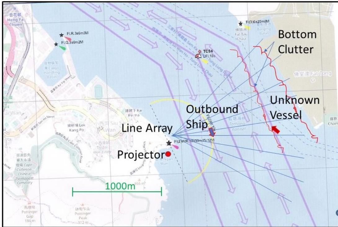
Figure 1: A notional system for ship channel monitoring
