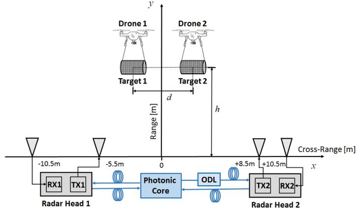
Figure 3. Geometry of the coherent photonics-based MIMO radar network and in-field experimental setup.
