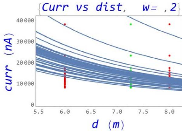
Figure 9 Collected current by photodiode for different Led stress vs distance in water ( $w=2$ ) and distance=7.1m. The red points are our, simulated, measurements. We try to match the curves: best result is for  $d=7.26$  m
