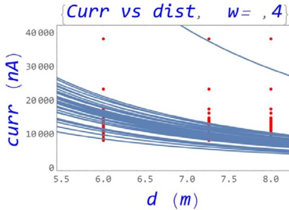
Figure 8 Collected current by photodiode for different Led stress vs distance in water ( $w=4$ ) and distance=7.1m. The red points are our, simulated, measurements. We try to match the curves without success
