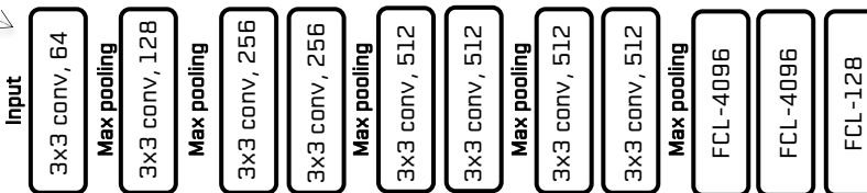
Architecture of VGGish network. The input size is 96x64 for log Mel spectrogram audio inputs
